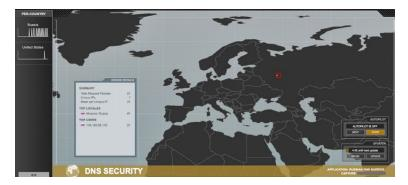
ExtraHop's Geomaps function can track real-time user activity by location to identify potential threats. The screenshot above shows DNS queries to IP addresses in Russia.
