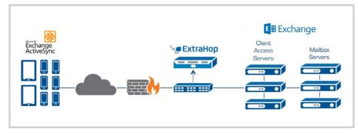
The ExtraHop platform deploys passively from a SPAN or network tap, equipping IT teams with a real-time view of communications. The above diagram illustrates how ExtraHop deploys to support Exchange ActiveSync projects.
