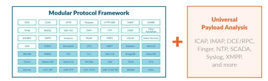
Universal payload analysis makes it possible to support virtually any protocol based on UDP or TCP.
