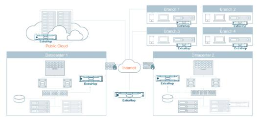
The ExtraHop Command appliance (ECA) provides an aggregated and unified view across hundreds of ExtraHop Discover appliance (EDA) nodes in different environments.
