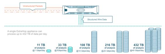
The ExtraHop platform performs stream analytics, transforming network packets into structured wire data in real time. This enables InfoSec teams to continuously analyze all east-west traffic and proactively detect bad actors.
